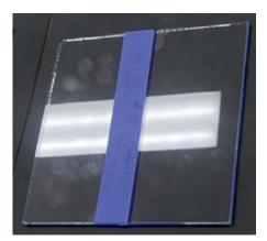
Left side of glass panel is uncoated while the right side is coated. The photo on the left shows fingerprints on both the uncoated and coated side. The same panel is photographed after 3 days. Fingerprints have significantly reduced on the coated side of the panel.
